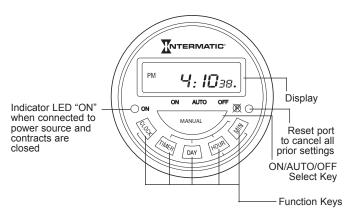
This electronic 7-day timer is accurate to the minute, and has the capcity to accept up to 16 set points (16 ON and 16 OFF times) and can be set to repeat the daily program 15 different ways:
